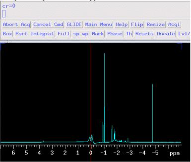
If you query "cr?" when the cursor is on the reference DSS line, you get a frequency value that assumes water is at 0.000 ppm, which is just the same as the frequency of water when DSS is set to 0.000 ppm, only negative. This is shown below.
